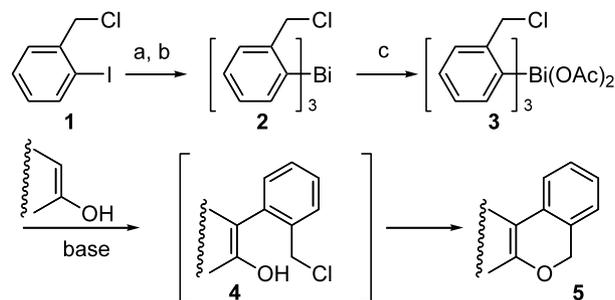
**Scheme 1.** Reagents and conditions: (a) *i*-PrMgBr, THF, –10 C, 3 h; (b) BiCl<sub>3</sub>, –10 C, 2 h, then rt overnight; (c) PhI(OAc)<sub>2</sub>, CH<sub>2</sub>Cl<sub>2</sub>.
